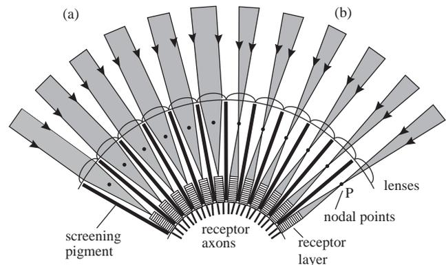
Fig. 2. Representations of Müller's theory. (a) A parallel beam is focused to a point in each ommatidium, as many authors supposed, with increasing gaps between the beams further from the eye. (b) A more realistic representation with the receptor projected through the nodal point and with sampling independent of range.
