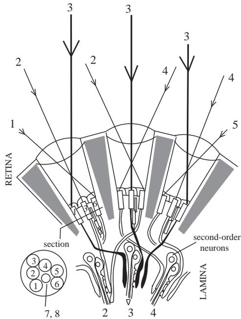
Fig. 6. The optics in higher Diptera, and perhaps some other open rhabdomere eyes. Behind each facet is a tiny fixed retina. The rays that are parallel outside the eye (with the same numbers) are directed to different receptors in adjacent ommatidia. They are recombined at the level of the second-order neurons by the appropriate paths of the retinula cell axons. Cells 7 and 8 lie on the central optical axis and their axons bypass the lamina.
