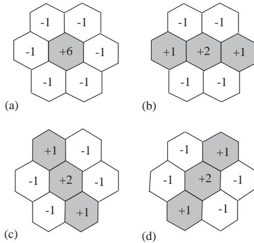
Fig. 13. Local filters for models of insect vision. (a) A hypothetical temporal modulation detector based on a hexagonal grid, as in the bee. (b–d) A set of three hypothetical orientation detectors that are compatible with data from the honey bee. These filters are similar to Canny detectors as used in machine vision.
