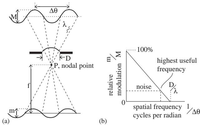
Fig. 5. The diffraction limit with an extended grating as object. (a) A sinusoidal grating of modulation  $M$  is focused by a lens of aperture  $D$  to an image with relative modulation  $m$ , given by  $m/M$  in (b). The relative modulation  $m/M$  is zero at  $\Delta\theta = \lambda/D$ , but the practical limit is set at a larger period by the noise level. Note that modulation detection does not involve perception of the pattern.
